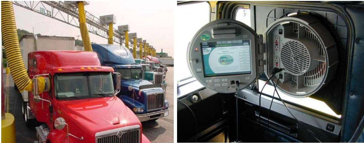
Figure 2. Photographs showing trucks using TSE as well as the console unit.
